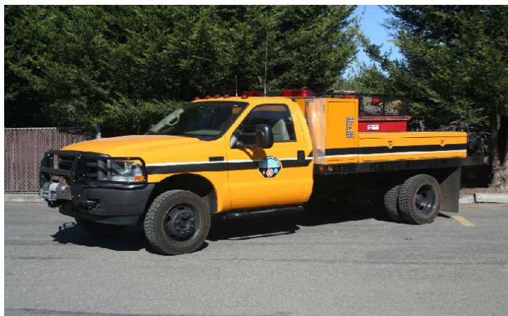
Example of a Brush Truck with Chassis
